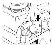
Slide the faucet valve assembly into 8. place on the hopper.
