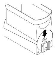
**8.** Remove the auger nose bushing **g**. from inside the hopper.
