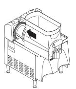
**4.** Thoroughly rinse the hopper(s) and install over the auger(s) and cooling drum(s).
