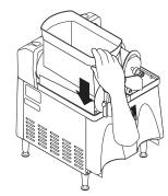
Slide into place and push down until 5. the hopper lock plunger(s) snap into place. On models with autofill, reconnect fill hoses and level probe to hopper.
