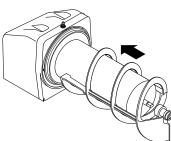
auger(s). Push the auger(s) as far as they will go and rotate so the flat face of the auger shaft is aligned with the flat face of the auger nose.
