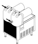
**3.** Remove the rear plastic plug from the trim strip between the hopper drip trays and loosen the auger motor cover screws.
