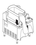
**12.** Slide the hopper(s) into place and push down until the hopper lock plunger snaps into place. For models without PAF, proceed to step 15.
