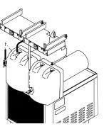
Place PAF platform assembly 5. on top of the motor covers and install support rod into hole in trim strip.
